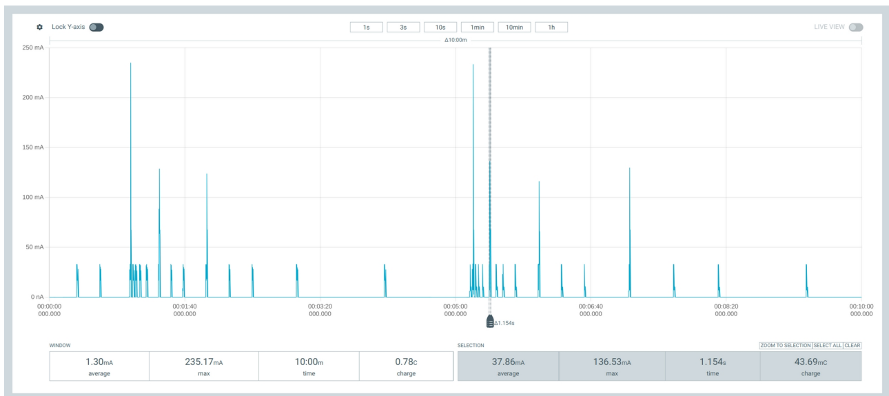
Fig 2.7 PPK2 10min diagram with low_power and high_power stages. Note low power (charge ~43.69mC) consumption for high_power stage with transmission due to the direct transmission of WiFi frames at MAC layer.
